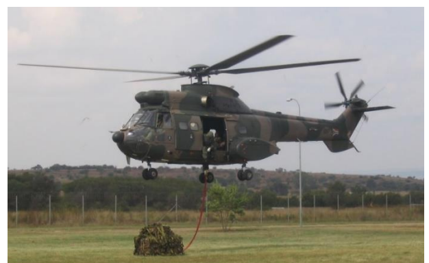
An Oryx preparing to lift an M5 mortar load
