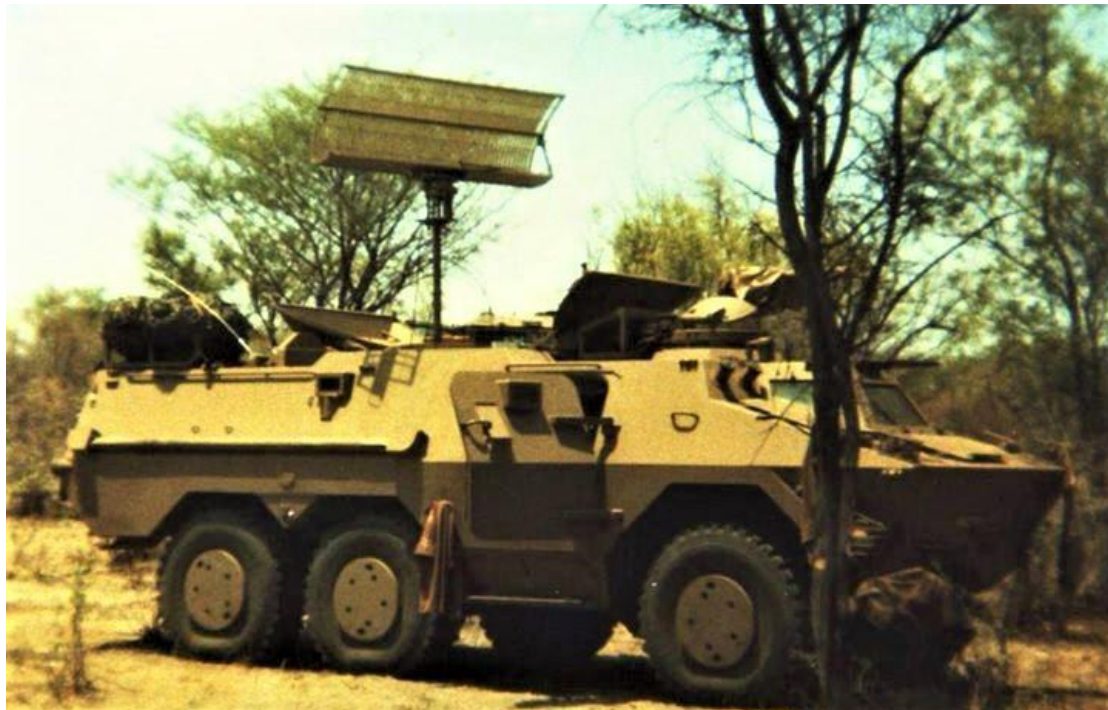
Figure 53: Example of Tupperware radar mounted on 81mm mortar Ratel vehicle
